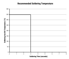
Soldering iron tip temperature should be set at 350°C (+10°C maximum), with the soldering duration not to exceed more than 3 seconds.
