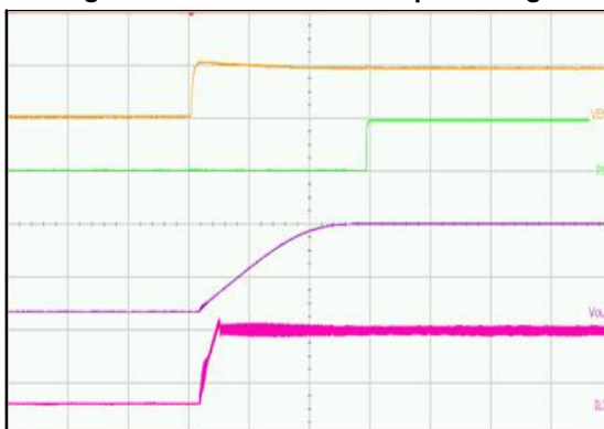
(VIN = 5 V, VOUT = 1.8 V, IOU = 3 A, CSS = 4.7 nF) Upper Trace: Enable Pin Voltage, 5 V / div Second Trace: Power Good Pin Voltage, 5 V / div Third Trace: Output Voltage, 2 V / div Lower Trace: Inductor Current, 2 A / div Time = 2 ms / div
