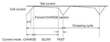
Charge mode continues until  $I_{COIL} \ge I_{REF}$ . After that the IC switches to SLOW DECAY mode and then switches to FAST DECAY mode for the last about 1 µs.
