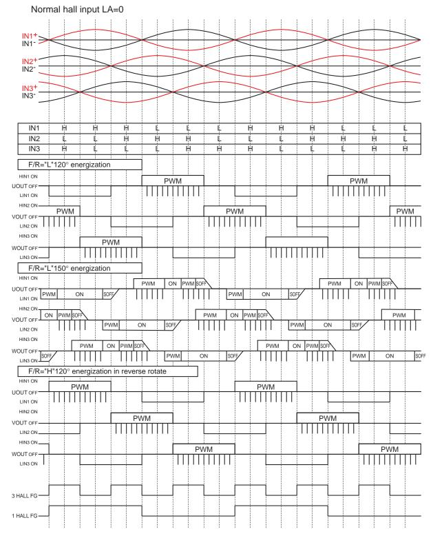
The energization is switched to 120° when 3 Hall FG frequency is 6.1Hz (TYP) or lower A direction of rotation is detected from Hall signal according to F/R pin input If the motor rotates in reverse against F/R pin input, 120° energization is maintained forcibly.
