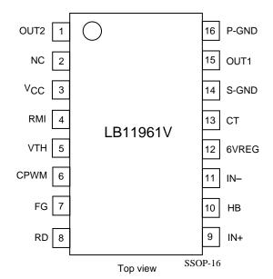
P-GND : Motor system ground S-GND : Control system ground
