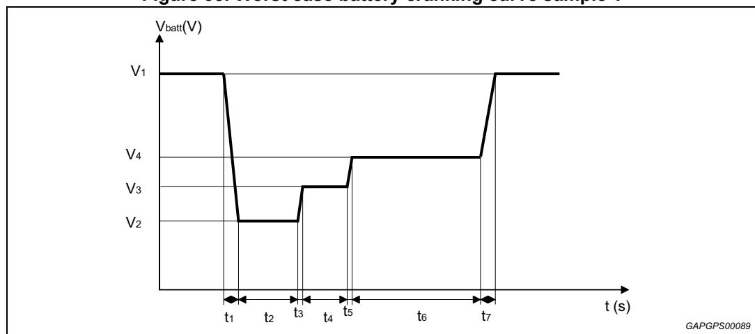
Figure 33. Worst case battery cranking curve sample 1
