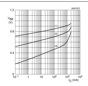
**TR1 (NPN);**  $V_{CE} = 5 \text{ V}.$
