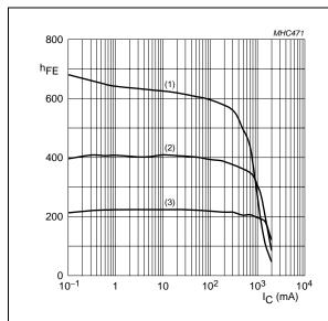
**TR1 (NPN);**  $V_{CE} = 5 \text{ V}.$
