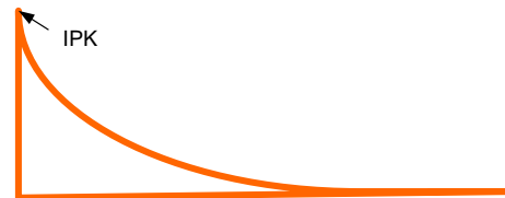
Figure 47. Input Charge Inrush Current
