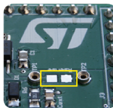
Figure 5. Pads for soldering SMD resistor
