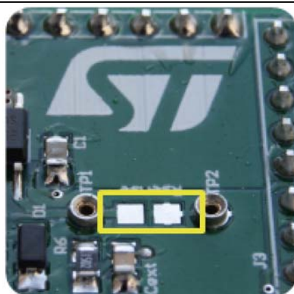
Figure 5. Pads for soldering SMD resistor
