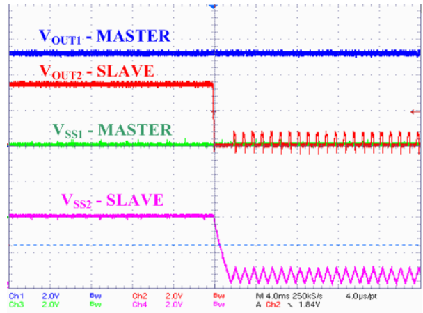
Figure 61. Master Voltage – End of Augmented OLM
