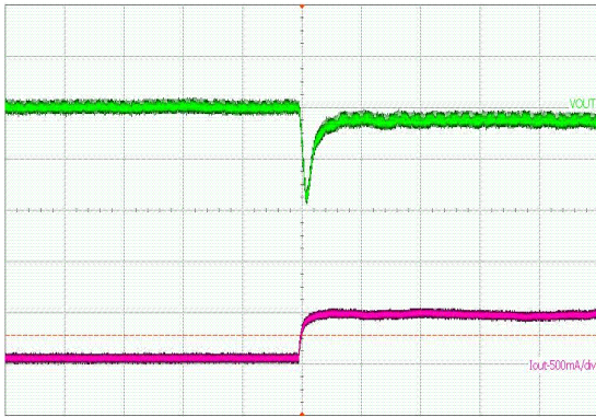
( V_{IN} = 5\text{ V} , I_{LOAD} = 100\text{ mA} , L = 3.3\text{ }\mu\text{H} , C_{OUT} = 2 \times 22\text{ }\mu\text{F} ) Upper Trace: Output Dynamic Voltage, 100 mV/div Lower Trace: Output Current, 500 mA/div Time Scale: 200 \mu\text{s}/\text{div}
