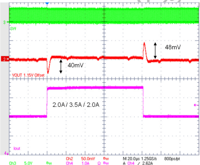
Figure 32. Transient Load 2.0 – 3.5 A Auto Mode
