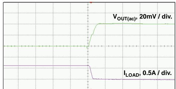
Figure 23. Fast Load Transient, Full Load to No Load
