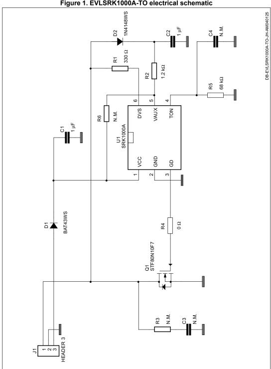
Figure 1. EVLSRK1000A-TO electrical schematic
