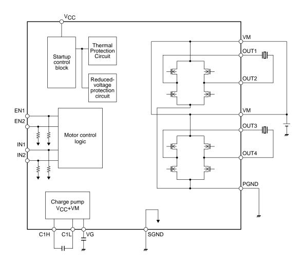
\* Connect a kickback absorption capacitor as near as possible to the IC. Coil kickback may cause increase in VM line voltage, and a voltage exceeding the maximum rating may be applied momentarily to the IC, which results in deterioration or damage of the IC
