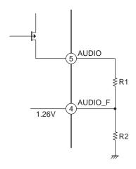
The AUDIO\_F voltage is determined by the internal band gap voltage of the IC (typ = 1.26V).
