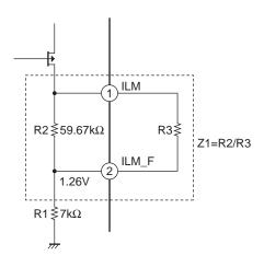
The ILM\_F voltage is determined by the internal band gap voltage of the IC (typ = 1.26V).
