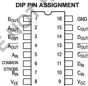
Pin assignment is for Dual-in-Line Package.
