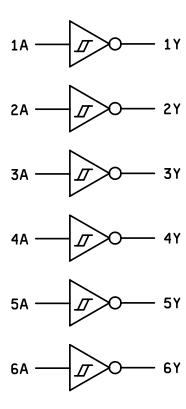
FIGURE 3. Logic diagram.
