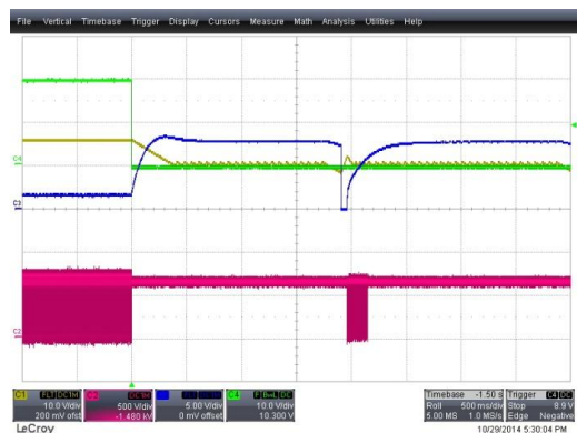
Figure 36. OLP Triggered, Output Short with 460 V AC , Full-Load, (CH1: V_{CC} (10 V/div), CH2: V_{DS} (500 V/div), CH3: V_{FB} (5 V/div), CH4: V_{OUT} (10 V/div), Time: 500 ms/div)
