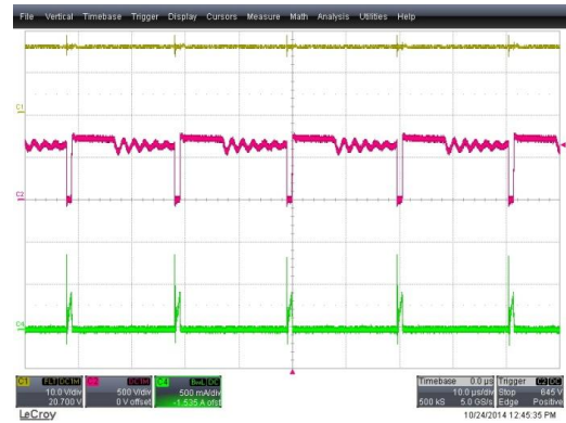
Figure 14. 460 V AC , Full-Load Condition (CH1: V CC (10 V/div), CH2: V DS (500 V/div), CH4: I DS (500 mA/div), Time: 10 \mu s/div)
