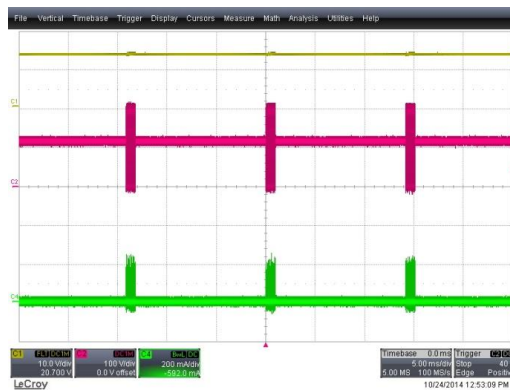
Figure 15. 85 V AC , No-Load Condition (CH1: V CC (10 V/div), CH2: V DS (100 V/div), CH4: I DS (200 mA/div), Time: 5 ms/div)
