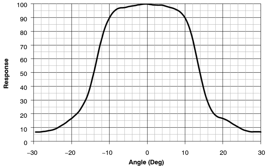
Figure 8. Monochrome with Microlens Angle Response
