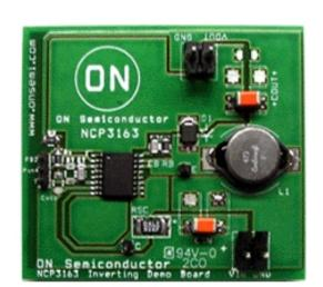
cycle oscillator with an active current limit circuit, driver and high current output switch. This controller was specifically designed to be incorporated in step -down, step -up, or voltage -inverting applications with a minimum number of external components. The NCP3163 comes in an exposed pad package which can greatly increase the power dissipation of the built in power switch.
