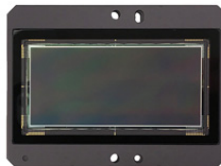
Figure 1. KAI-50140 CCD Image Sensor
