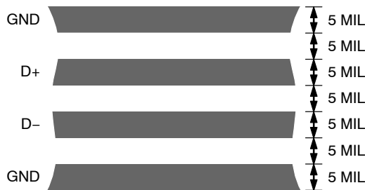
Figure 16. Typical Arrangement of Signal Tracks
