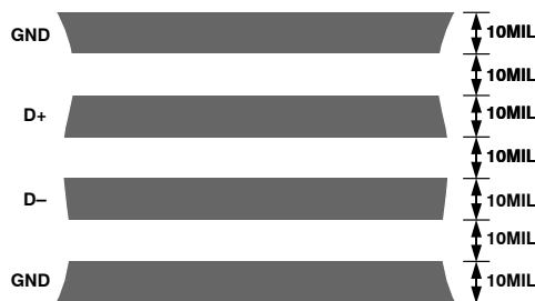
Figure 34. Arrangement of Signal Tracks
