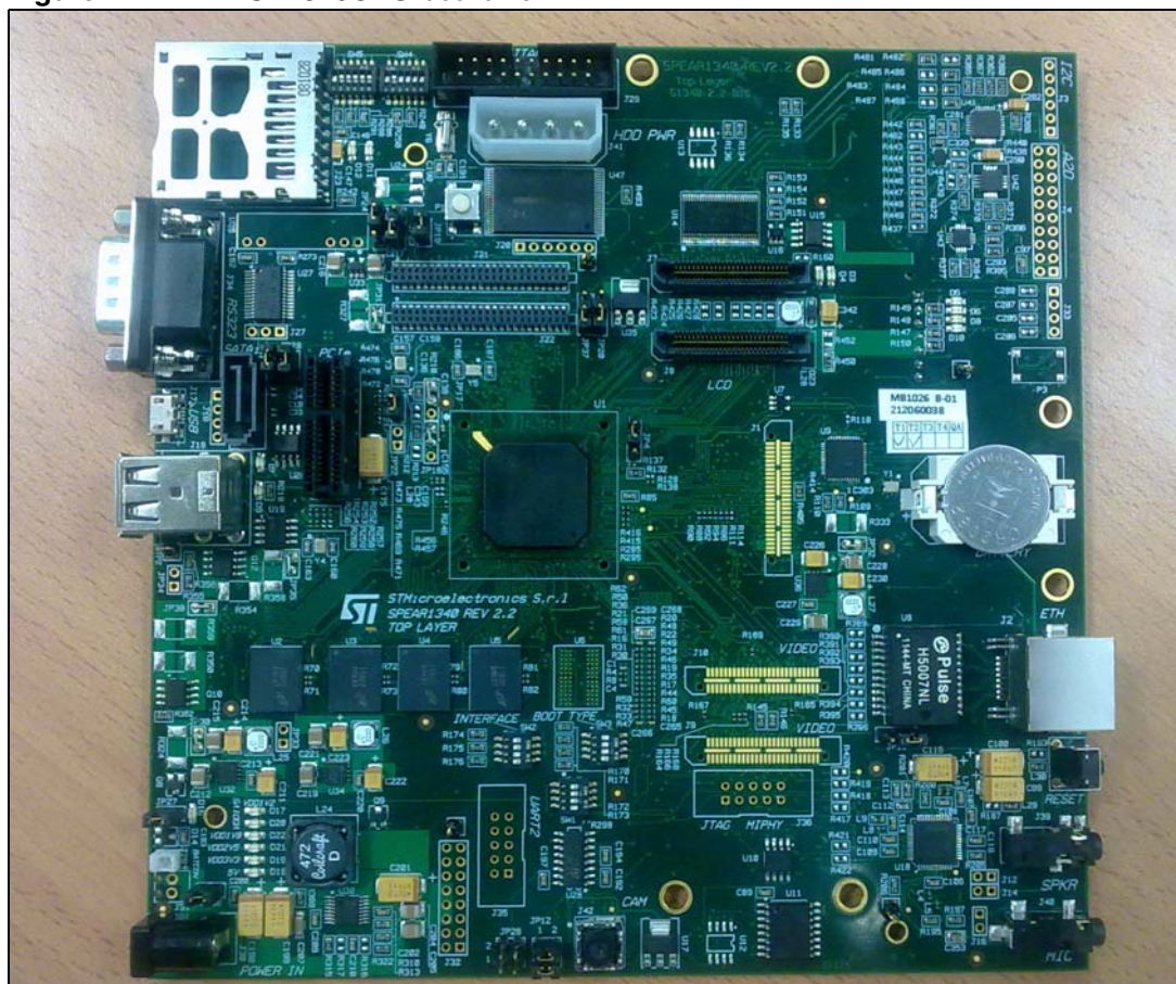
Figure 1. EVALSP1340CPU board rev. 2.2
