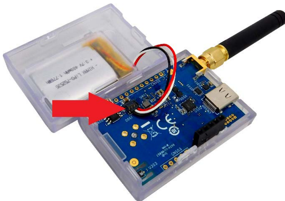
Figure 6. STEVAL-STRKT01 setup (3 of 4)
