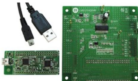
This kit makes it possible to operate the LSI evaluation board on your PC easily and quickly. We provide the board with the Daughter Board and the GUI that you can download from this site using the software link below.
