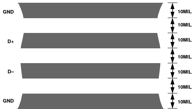
Figure 18. Typical Arrangement of Signal Tracks
