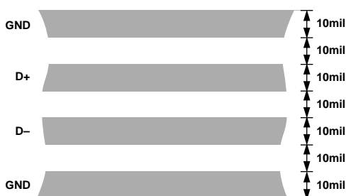
Figure 14. Arrangement of Signal Tracks
