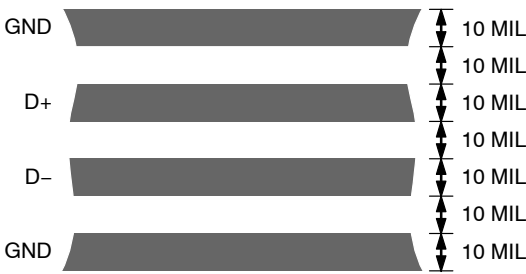
Figure 15. Arrangement of Signal Tracks
