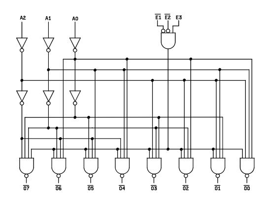
FIGURE 3. Logic diagram.
