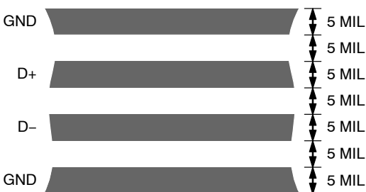
Figure 22. Typical Arrangement of Signal Tracks
