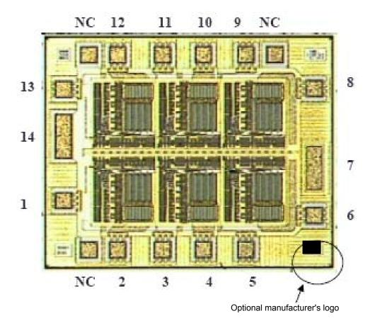
Pad size: Pad numbers 1 to 6 and 8 to 13: 100 x 100  $\mu$ m Pad numbers 7 (GND) and 14 (V<sub>CC</sub>): 100 x 280  $\mu$ m
