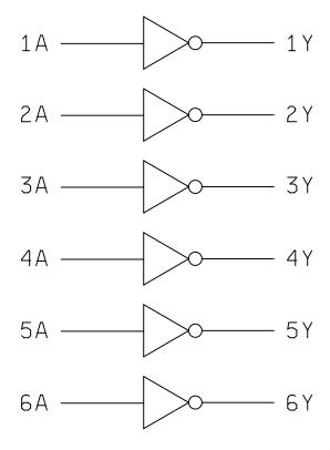
FIGURE 3. Logic diagram.
