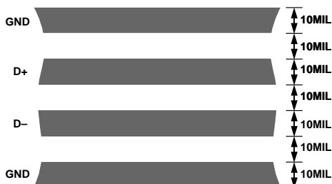
Figure 18. Arrangement of Signal Tracks
