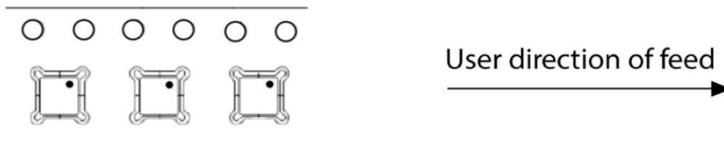
Figure 29. Package orientation in carrier tape
