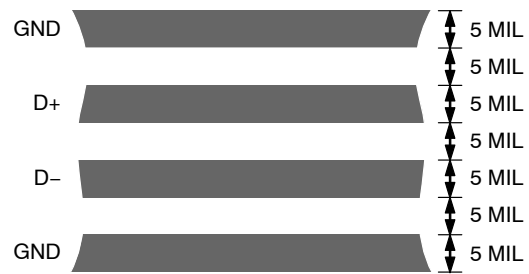
Figure 22. Typical Arrangement of Signal Tracks
