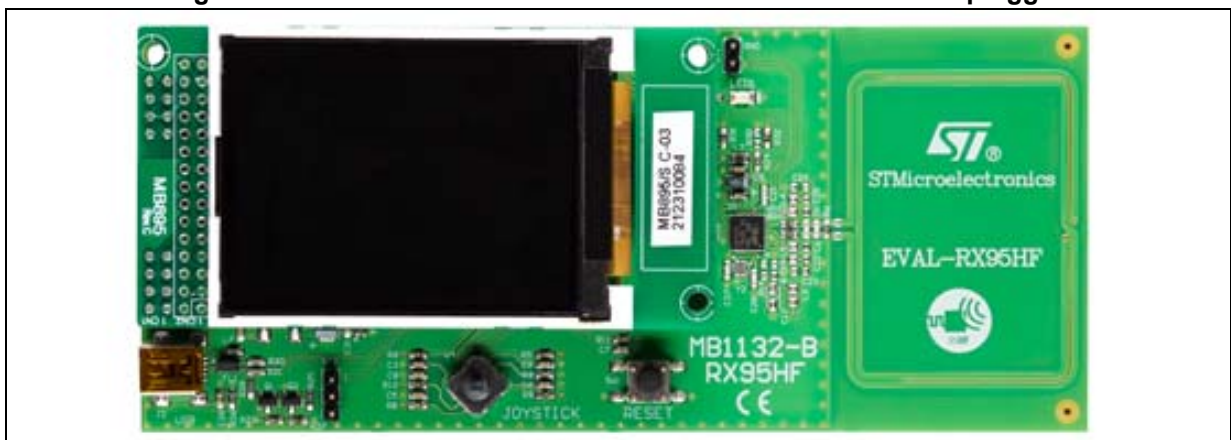
Figure 2. EVAL-RX95HF RF transceiver board with LCD screen plugged
