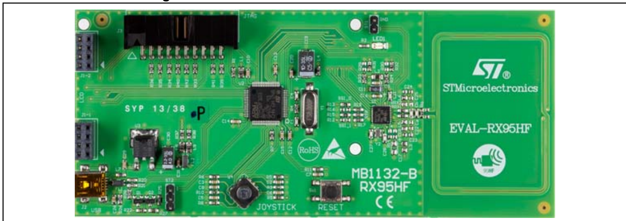
Figure 1. EVAL-RX95HF RF transceiver board alone
