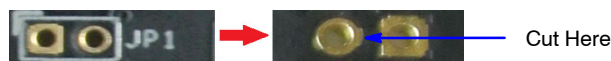
Figure 7. Top and Bottom View of Shorted Jumper. The Bottom View Shows the Trace Location to Cut for Current Measurement
