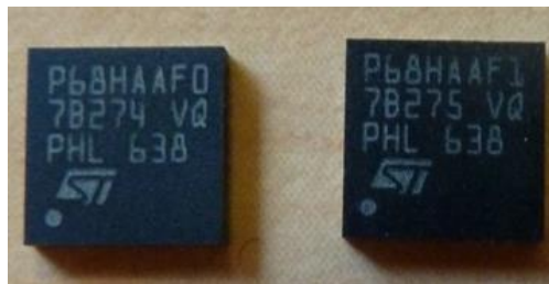
Figure 2: Picture of the Cryptographic Module (VQFN32) – Marking
