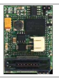
SPC563MxxAVBx Vertical base board for SPC563x line and moreover the board enables the use of new enhanced automotive calibration and debug tools on the SPC563Mx line of automotive microcontrollers, featuring a 16-bit bus interface.
