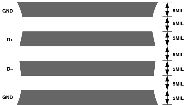
Figure 16. Typical Arrangement of Signal Tracks
