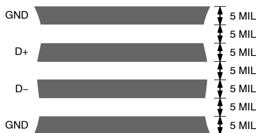
Figure 21. Typical Arrangement of Signal Tracks
