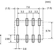
Tolerance of lead pitch is  $\pm 0.15 \text{mm}$  (0.006inch) Other tolerances  $\pm 0.3 \text{mm}$  (0.012inch) Coplanarity of terminals is 0.1mm Max.
