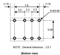
Tolerance of lead pitch is  $\pm 0.15 \text{mm}$  (0.006inch) Other tolerances  $\pm 0.3 \text{mm}$  (0.012inch)
