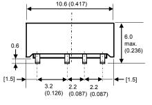
Tolerance of lead pitch is  $\pm 0.15$ mm (0.006inch) Other tolerances  $\pm 0.3$ mm (0.012inch) Coplanarity of terminals is 0.1mm Max.
