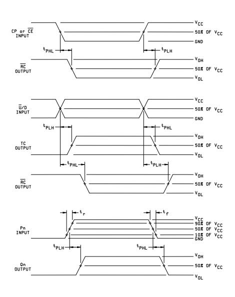
FIGURE 4. Switching waveforms and test circuit – Continued.
