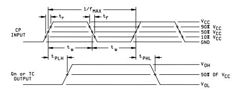
FIGURE 4. Switching waveforms and test circuit.
