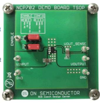
A Logic EN input provides ON/OFF control of the output voltage. When the EN is low the device consumes as low as typ. 10nA from the IN terminal. The device is fully protected in case of output overload, output short circuit condition and overheating assuring a very robust design.
