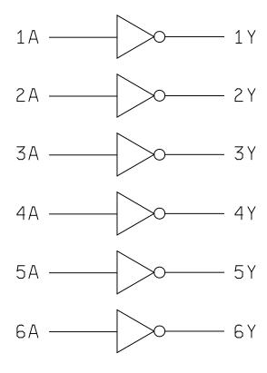
FIGURE 3. Logic diagram.
