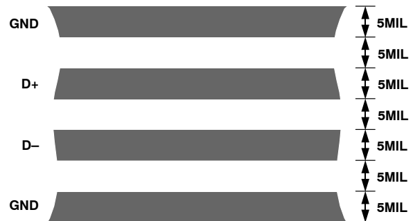
Figure 21. Typical Arrangement of Signal Tracks
