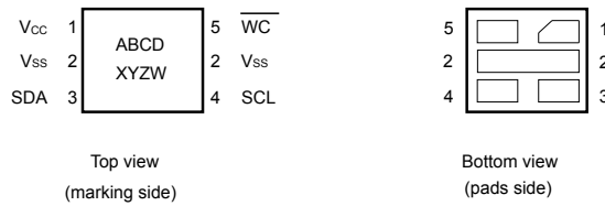
Figure 3. UDFPN5 (DFN5) package connections
