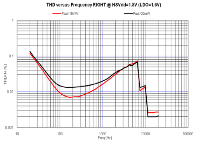
Figure 12. THD+N vs Frequency, 32 \Omega Load in Phase, Right Channel
